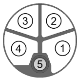
Fig. 2: Motor. L-coded M12 (m).
