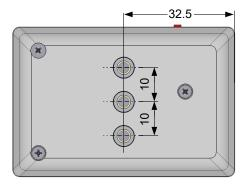
Alternatively, you can also screw on a DIN rail clip and install the adapter in a switch cabinet.
