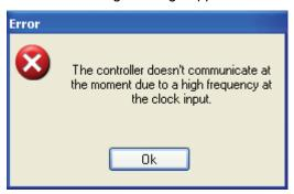
Communication can only take place again if a clock frequency of less than 65 kHz is set.
