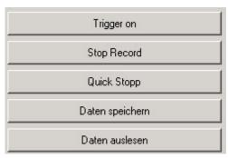
The <Test Record> button changes to the <Trigger on> button: When this button is clicked, the trigger signal is set and the motor changes from the Speed mode to the Relative positioning mode.
