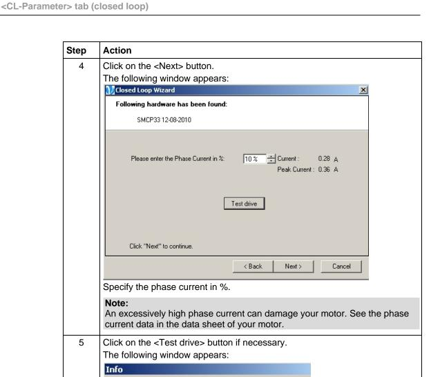
Click on the <Ok> button: An attempt is made to move the motor by one rotation using the specified parameters.
