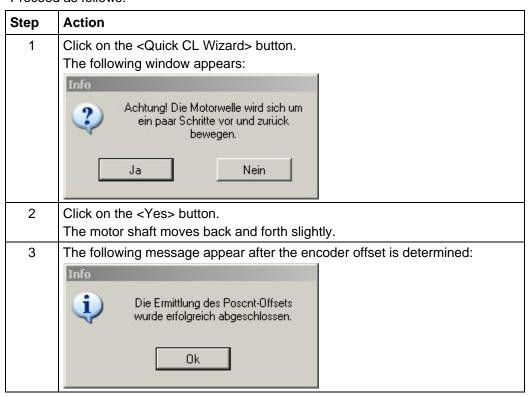
The encoder offset is only determined if the value is "0" before the quick test run. Otherwise, the shaft does not move and a value is not determined.
