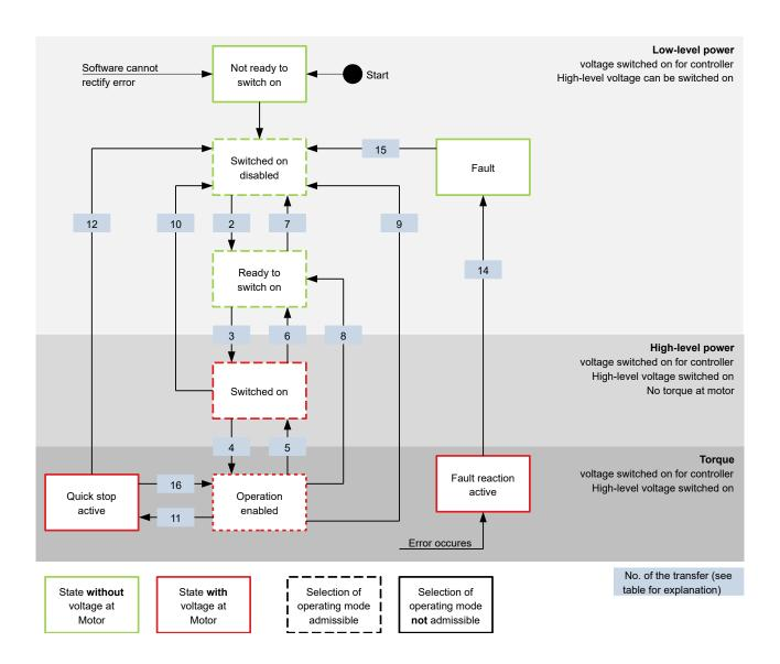
Listed in the following table are the bit combinations for the controlword that result in the corresponding state transitions. An X here corresponds to a bit state that requires no further consideration. Exceptions are the resetting of the error (fault reset) and the changeover from *Quick Stop Active* to *Operation Enabled*: the transition is only requested by the rising edge of the bit.
