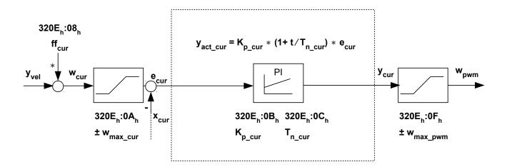
For each controller you can set a maximum control deviation ( $e_{max}$ ) and a *gain factor* ( $K_p$ ) that determine the output of the controller (control variable), taking into account the limitation of the control variable ( $y_{max}$ ).
