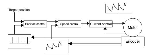
In the *slow speed* mode, the motor instead operates with constant phase current, as in *open loop*. The following error is, however, monitored by means of the encoder and the vector control of the magnetic field is activated if necessary, as in *closed loop*.
