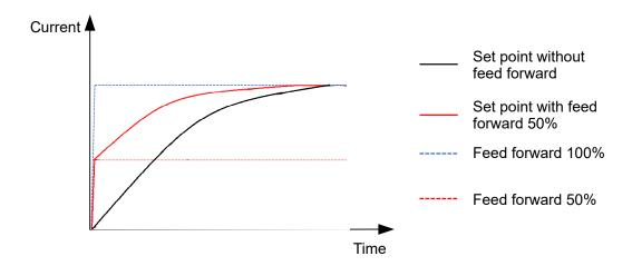
The factor for the *velocity feed forward* is set in object  $320E_h$ :03<sub>h</sub> in tenths of a percent of the output of the ramp generator ( $606B_h$ ) and added to the output of the position controller before the velocity controller. The *velocity feed forward* is active in all modes with position control loop:
