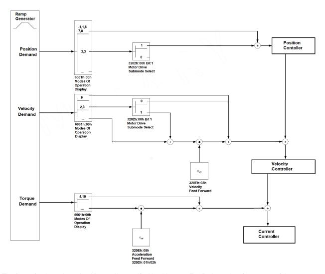
The factor for the *voltage feed forward* is specified in object  $320E_h$ :0D<sub>h</sub> in tenths of a percent of the voltage that is needed to produce the rated current. If the factor is 1000‰ (factory setting), the voltage is immediately available and the actual current quickly reaches the rated current. As a result, there is practically no control deviation during acceleration and the current controller is relieved.
