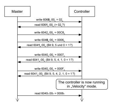
**4.** To stop the motor, set controlword (6040<sub>h</sub>) to "6".
