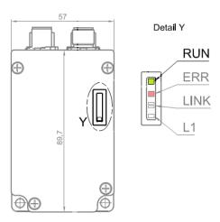
The green RUN LED indicates one of the following controller states (EtherCAT slave):
