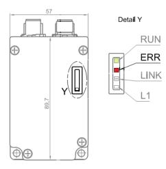
The red ERR LED indicates one of the following controller states (EtherCAT slave):
