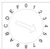
The NodeID can either be applied as a value from the adjuster wheel or read from object **2009 h**.
