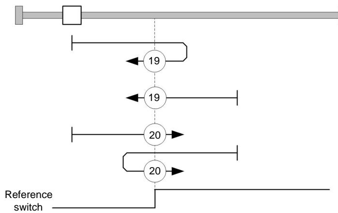
In the methods 21 and 22 (equivalent to methods 5 and 6), the right switch flank of the reference switch is used as a reference:
