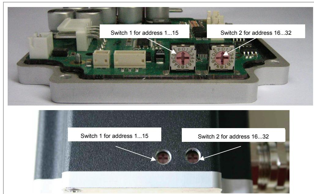
The 1st digit is set with switch 1 (left), the 16th digit of the address is set with switch 2 (right).
