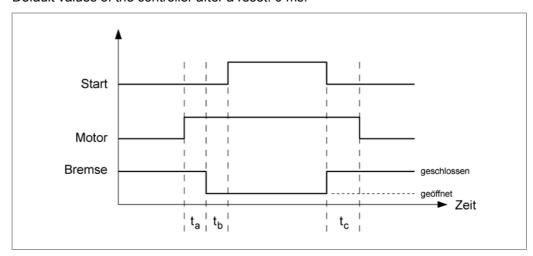
When switching on the controller, the brake becomes active first and the motor is not provided with power. First the motor current is switched on and a period of ta ms waited. Then the brake is disengaged and a period of tb ms waited. Travel commands will only be executed after expiry of ta and tb.
