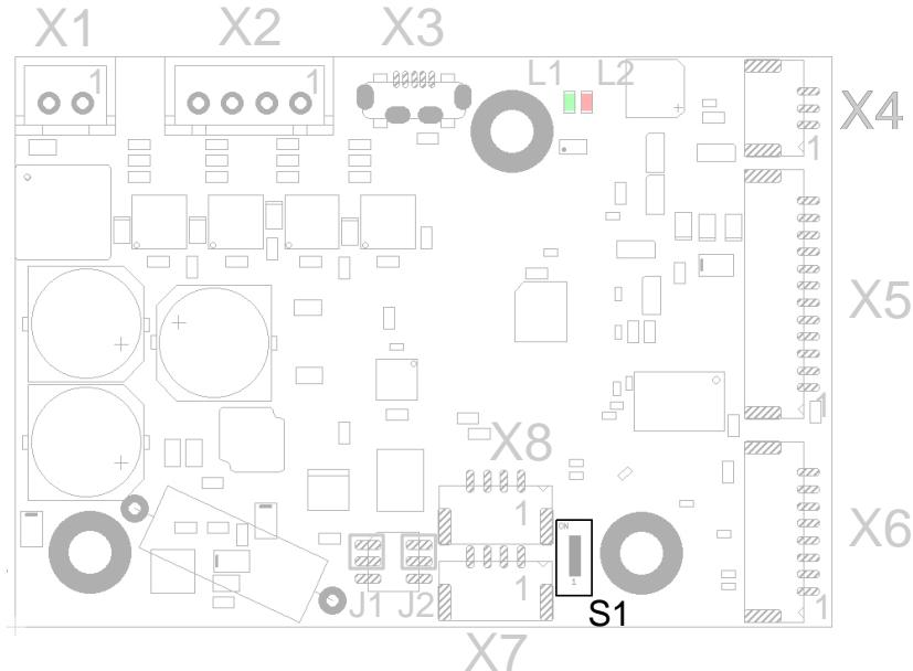
With this switch a terminating resistor of 120 ohm can be switched in between CAN\_L and CAN\_H, or RS485- and RS485+, on or off.
