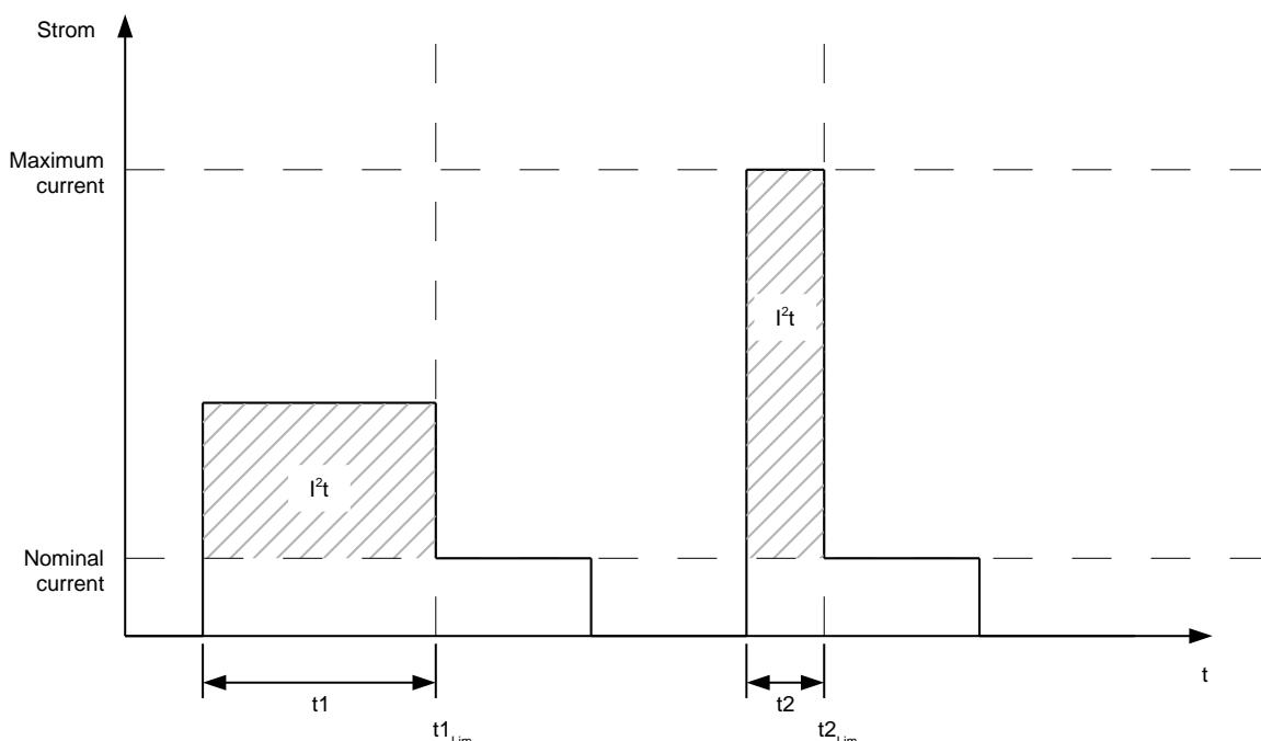
In the first section  $t_1$ , the current value is higher than the nominal current. At time  $t_{1,Lim}$ ,  $I^2t_{Lim}$  is reached and the current is limited to the nominal current. During the following time period  $t_2$ , a current comes that corresponds to the maximum current. Accordingly, the value for  $I^2t_{Lim}$  is reached faster than in time period  $t_1$ .
