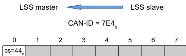
**Byte 0 : CS (Command Specifier)**Wert = "44<sub>h</sub>"**Bytes 1-7 :**reserviert (=0<sub>h</sub>)**8.3.3.2 Configuration services**
