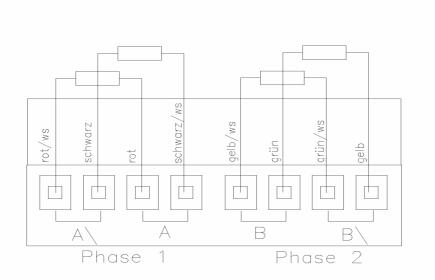
Motors with 8 leads are connected internal parallel.
