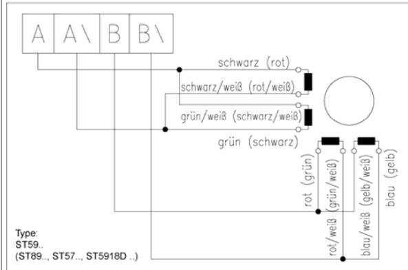
**8 lead wire - serial for low frequency < 1 kHz**
