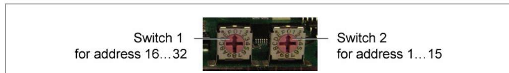
The 16's place is set with switch 1 (left) and the 1's place is set with switch 2 (right).
