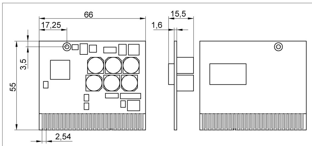
**SMCP33-K dimensions (with heat sink)**
