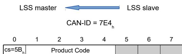
**Byte 0 : CS (Command Specifier)**Wert = "5B<sub>h</sub>"**Bytes 1-4: Product Code**Product Code: siehe 1018<sub>h</sub>:02<sub>h</sub>**Bytes 5-7 :**reserviert (=0<sub>h</sub>)**3. Der LSS-Master fragt die Revision Number ab:**
