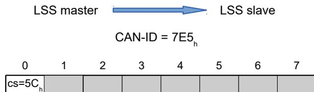
**Byte 0 : CS (Command Specifier)**Wert = "5C<sub>h</sub>"
