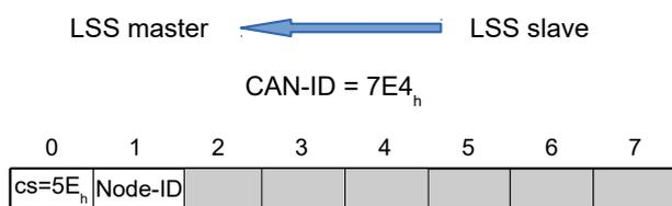
**Byte 0 : CS (Command Specifier)**Wert = "5E<sub>h</sub>"**Byte 1: Node-ID**
