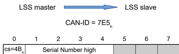
**Byte 0 : CS (Command Specifier)**Wert = "4B<sub>h</sub>"
