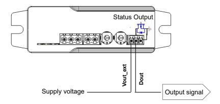
The output signals the state of the brake chopper: as long as the output is HIGH (( $D_{out}=V_{out\_ext}$ ), the supply voltage ( $U_p$ ) is available and no errors have occured. If the output turns LOW ( $D_{out}=GND$ ), an error has occured. The red LED signals the exact error number,
