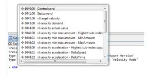
This also works if you need the index of an object where you know the name of an object. Start by typing in the name (for example "Statusword") and press **Ctrl** and **Space** and select the entry of interest as described in the example above.
