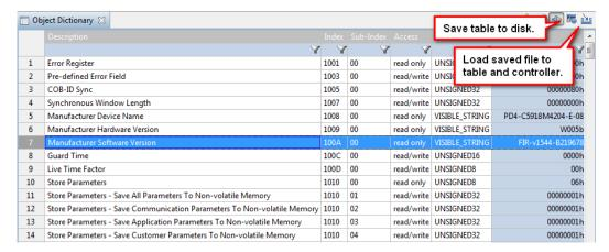
The file uses the same format as the Object Dictionary Script Console. So as an alternative for loading the file, it is possible to copy the content - or parts of it - to the Object Dictionary Script Console.
